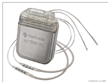
Modern Activa PC neurostimulator Courtesy of Medtronic, Frans Gielen
