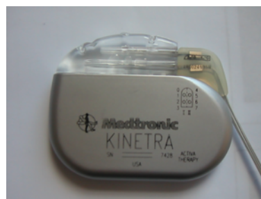
Modern Activa PC neurostimulator Courtesy of Medtronic, Frans Gielen
